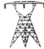
115 kV Steel Lattice Average height 75' Average span 1150'
