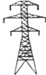
230 kV Steel Lattice Double Circuit Average height 120' Average span 1150'
