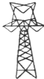
500 kV Lattice Average height 125' Average span 1150'
