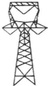
500 kV Lattice Average height 135' Average span 1150'
